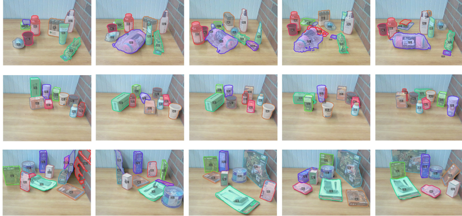
Figure 5: Visualized results for the table environment. Masks with the same color and index are associated and predicted as the same object by the network.
